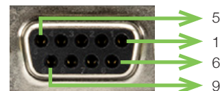
Figure 14. RS232 pin numbering
