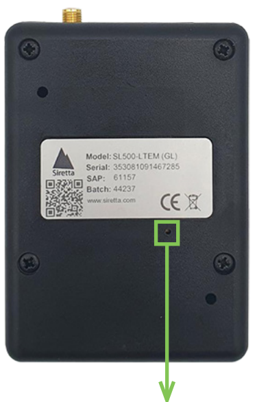
SL500 modem configuration function boot switch
