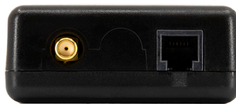
Figure 11. SL500 Modem - Antenna and Power Connector
