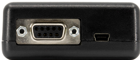
Figure 10. SL500 Modem - RS232 and USB Ports
